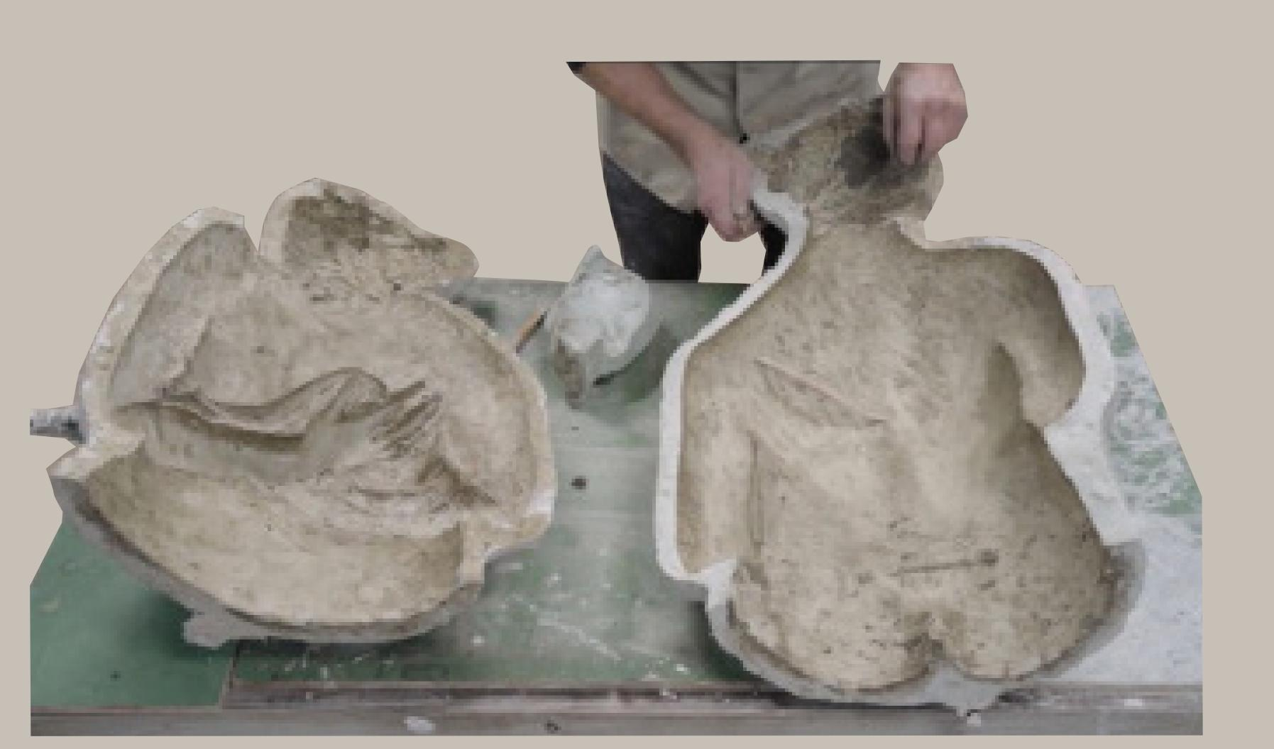
Fig. 6. Two sections of a plaster mold
