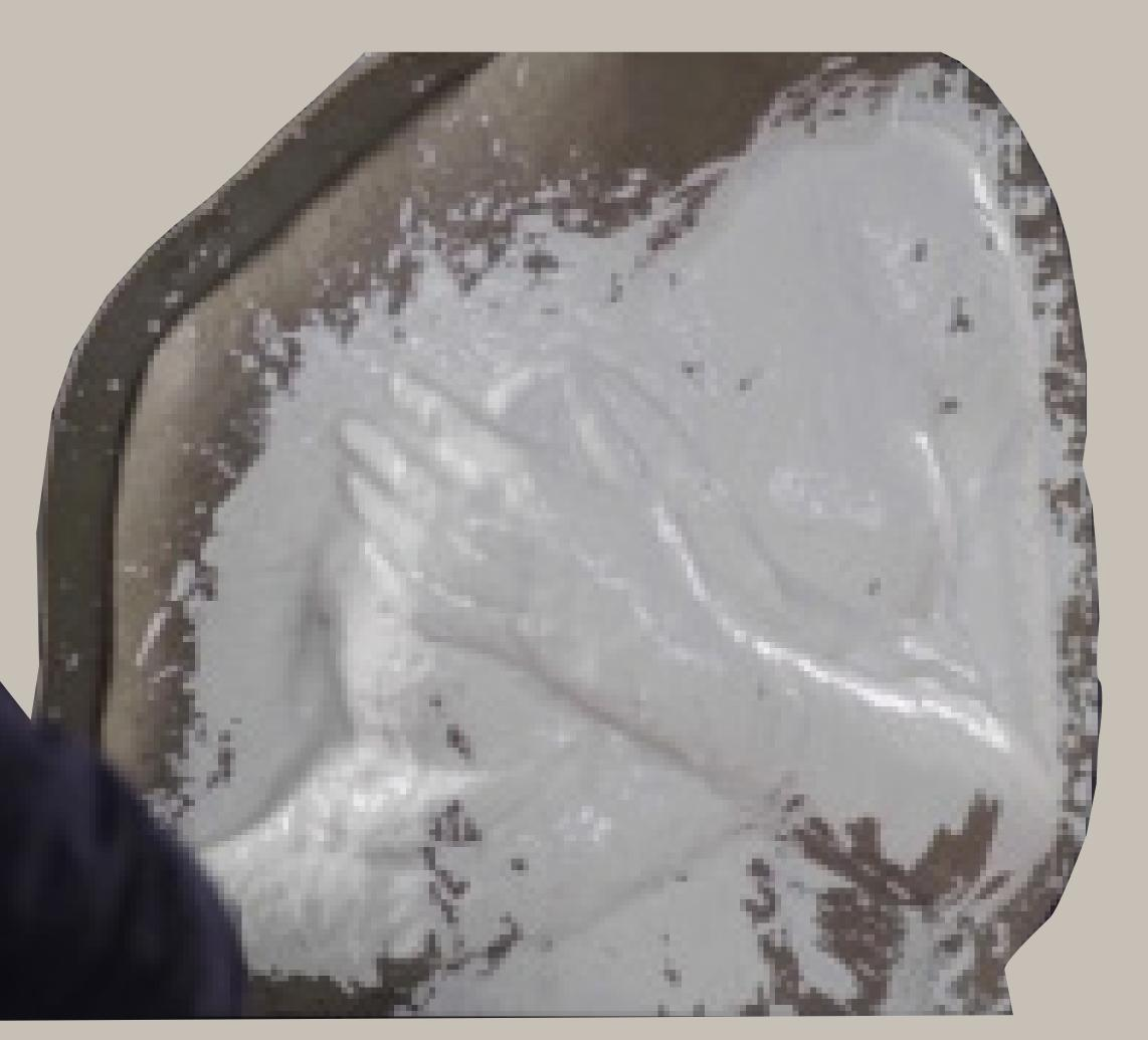
Fig. 5. Coating a clay model with plaster
