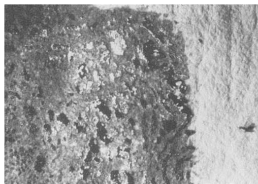
31. Detail, fig. 30, showing pigment particles scattered in the thin resin layer
